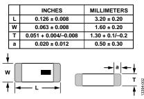
Figure 2. Mechanical Dimensions
