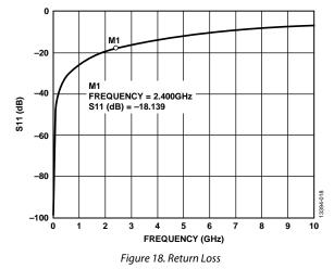
Return loss characterizes the amount of power reflected from the feed line and is a commonly valued parameter for the antenna. It is usually displayed as S11 in dB. Figure 19 indicates that the RF radiates at 2.400 GHz, with S11 = -18.139 dB. It is more efficient than the acceptable return loss of -10 dB to -15 dB and reflects only 1.58% of the power.
