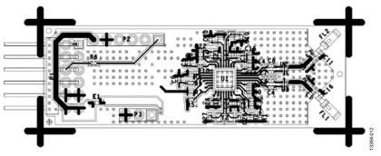
Figure 12. EVAL-ADF7242-PMDZ Board Layout Highlighting the Chip Antenna Placement
