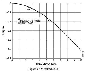
Acceptable insertion loss for the PCB layout is less than 1 dB. Maximize the allowable insertion loss of the PCB to optimize the RF performance. Figure 19 indicates that an insertion loss of -0.084 dB has a minimal effect on the power transferred.
