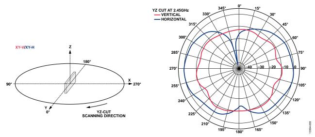
Figure 9. 2450AT18A100 Chip Antenna Typical Radiation Pattern, YZ Cut at 2.4 GHz (25°C)
