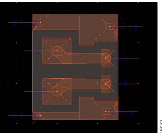
Figure 15. Trace from Decoupling Capacitor to Balun Balanced Port
