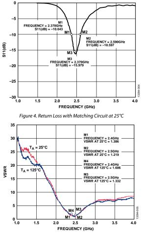
Figure 5. VSWR with Matching Circuit at 25°C and 125°C
