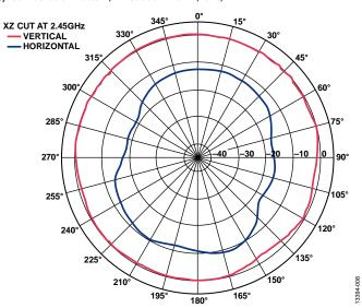
Figure 8. 2450AT18A100 Chip Antenna Typical Radiation Pattern, XZ Cut at 2.4 GHz (25°C)
