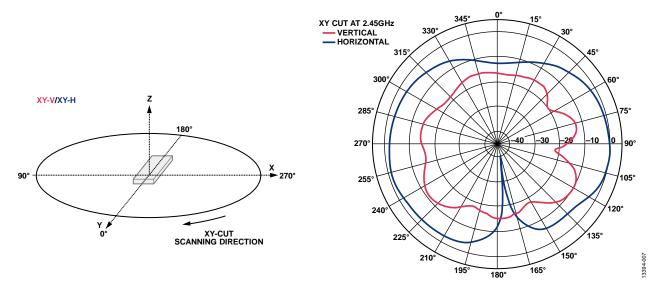
Figure 7. 2450AT18A100 Chip Antenna Typical Radiation Pattern, XY Cut at 2.4 GHz (25°C)
