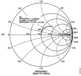
Figure 20. Corresponding Impedance Measurements
