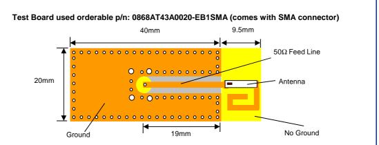
Note: It is recommended that the designer leave available slots for a "pi" (or shunt-seriesshunt) network. The antenna matching network values above are used when antenna is monted on Johanson's evaluation board. The matching values on clinet's PCB will be different. Go to: www.johansontechnology.com/tuning and see how to obtain the new values. If you need further help, contact our RF Applications Eng Team at: www.johansontechnology.com/ask-a-question
